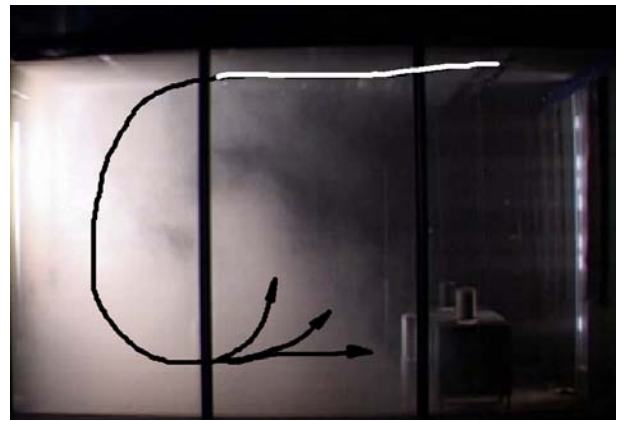
Room air flow visualization possible in the LTG lab (LTG Engineering Services)
