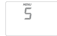
keep pressing MENU button until seeing 0 transmitter is not working in MENU mode
